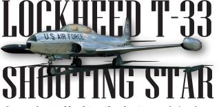
The two-place **Lockheed T-33 Shooting Star** was designed for training pilots already qualified to fly propeller-driven aircraft. It was developed from the single-seat F-80 fighter by lengthening the fuselage about three feet to accommodate a second cockpit. In addition to its use as a trainer, the T-33 has been used for such tasks as drone director and target towing, and in some countries even as a combat aircraft.
