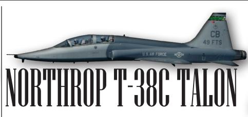
The **Northrop T-38C Talon** is a twin-engine, high-altitude, supersonic jet trainer used in a variety of roles because of its design, economy of operations, ease of maintenance, high performance and exceptional safety record. The T-38C model includes upgrades to the avionics systems including the incorporation of a "glass cockpit."Air Education and Training Command is the primary user of the T-38C for joint specialized undergraduate pilot training.
